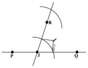
• Move the compasses to where the upper arc crosses the transversal line and draw an arc to make point *S*.
