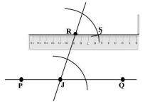
• The construction is complete. The line *RS* is parallel to *PQ*
