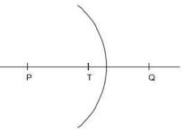
• Using the same radius and point *Q* as centre, draw an arc that intersects the first arc. Label the points where the 2 arcs intersect as *C* and *D*.
